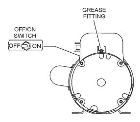
Figure 7. Single Phase Electric Motor with 12 inch Pigtail Cable
